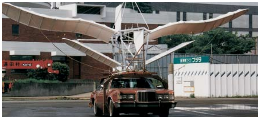
The Jewel Bug replica at Nihon University in 1991 testing the aerodynamics using a car instead of a wind tunnel
