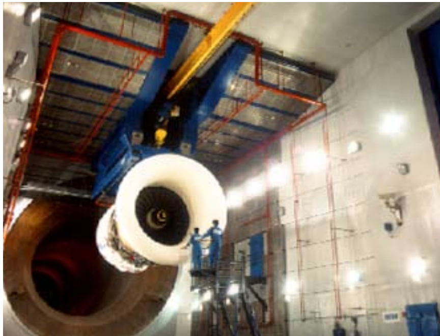
HAESL technicians inspect a Rolls-Royce Trent 800 engine in its Hong Kong test cell
