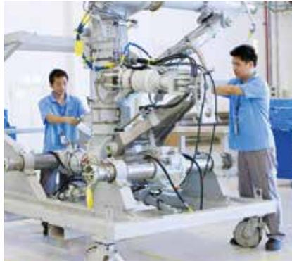
aircraft engine MRO specializes in quick-turn repairs and lease returns for commercial aircraft engines.
